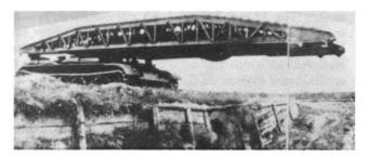
Figure 6-47. Tank-launched bridges. Two class-50 short-span bridges are used. The T-54 MTU (above) has a span of about 40 ft., while the (T-55) MTU-20 (below), with fold-up ramps at each end, has a span of about 68 feet.
